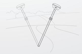
T10 supports NFC fast connection, you can automatically connected with data collector just a touch. It has multiple high-end connectivity modules including Bluetooth, Wi-Fi, NFC, and UHF radio modem. The internal LorRa UHF allows super-long-distance working range up to 15 km, making it working easier within RTK networks.
